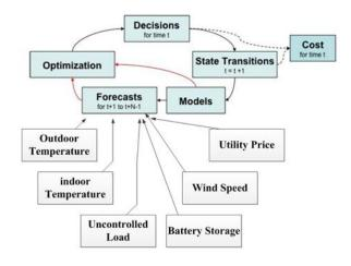
Figure 2: Load Forecasting Model.
