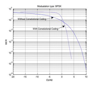
Fig. 1. BER vs Eb/N0 for Hamming Code and Convolutional Code.
