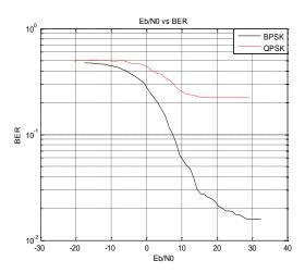
Fig. 2. Eb/N0 vs BER using BPSK, QPSK Modulation, Hamming code and interleaving.
