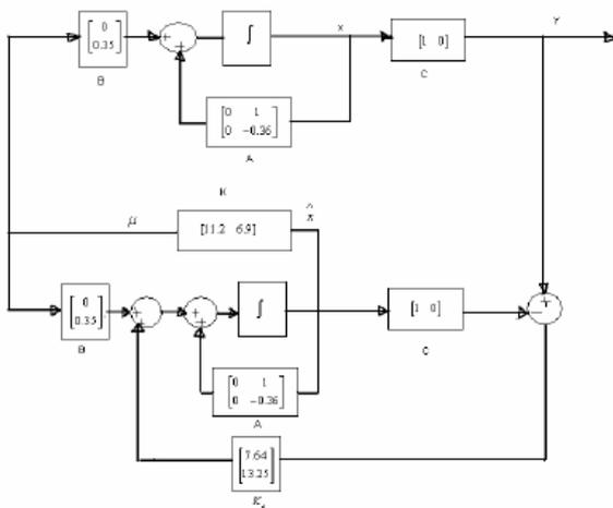
Fig.9 Simulation diagram of close loop control system with state observer.
