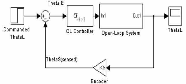
Fig.5 Closed loop feedback control diagram
