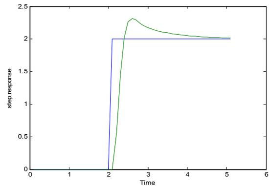
Fig.6b step response using ql compensator
