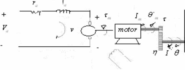
Fig.1 Model of a DC torque motor connected through gearing to an inertia load
