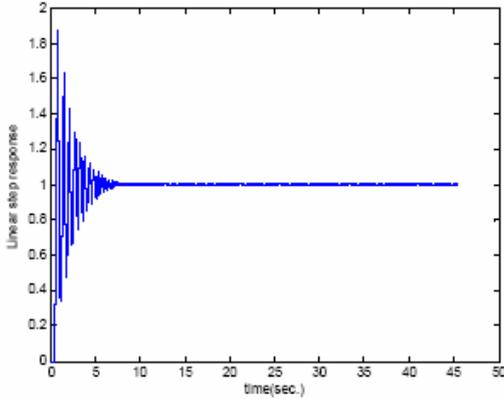
Fig.3 Response of the closed loop system with a linear compensator
