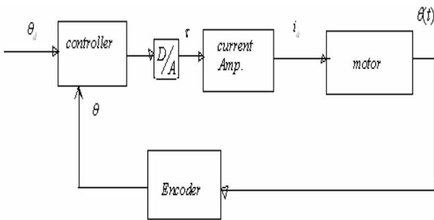
Fig.2 Block diagram of the robot joint-control system
