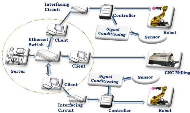
Fig.1. Block Diagram of DCS Based Micro-factory communicate between the server computer and client computers. For the “Robots and Multiple Sensor Management” portion, it is to build the pick and place three degree of freedom robot and its driver control circuits. And also the interface circuit between the computer and controller must be constructed.
