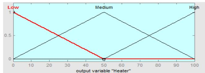
Fig. 6. Graphs of MFs for the Output Variable “Heater”
