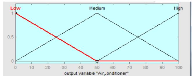
Fig. 5. Graphs of MFs for the Output Variable “Air Conditioner”
