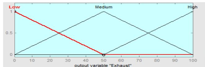
Fig. 7. Graphs of MFs for the Output Variable “Exhaust”
