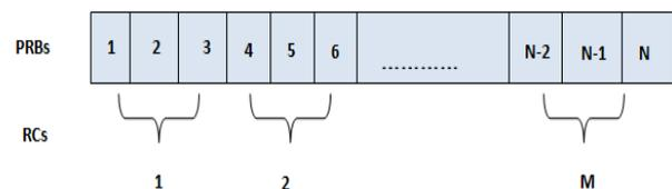
Fig 1: A total of M RCs dividing the total bandwidth into N PRBs.
