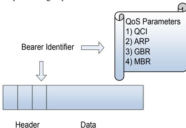
Fig 2: Packet format in LTE-A.
