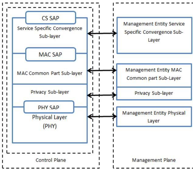
Fig. 1 Reference model of WiMAX MAC
