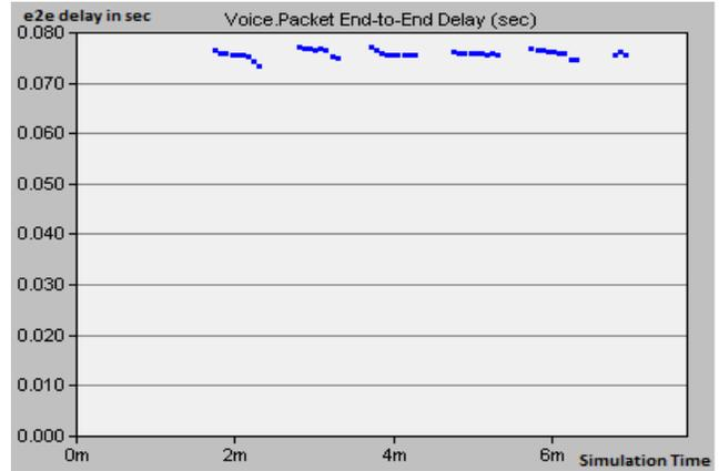
Fig. 3a Voice Packet end-to-end Delay Optimized for voice
