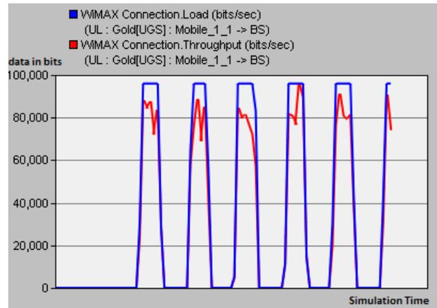
Fig. 3b WiMAX Connection Load vs. Throughput- Optimized for voice
