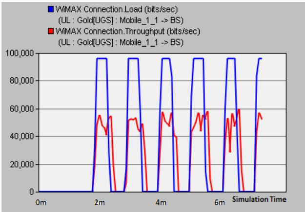
Fig. 2a WiMAX Connection Load vs. Throughput (Pre-optimization)
