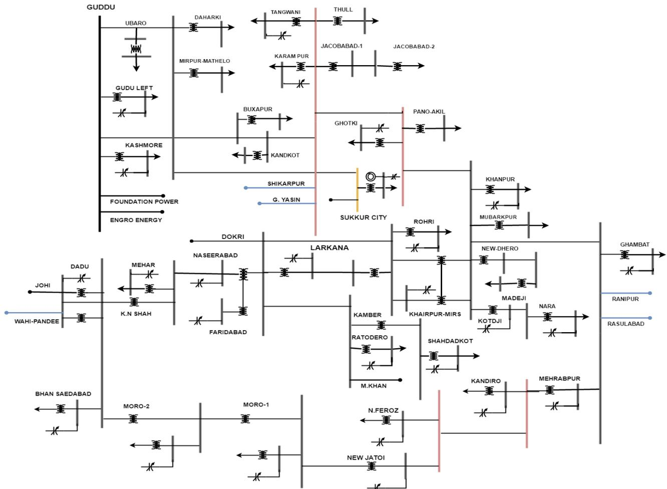
Fig. 1 One-line diagram of SEPCO network generated by E- Simulation
