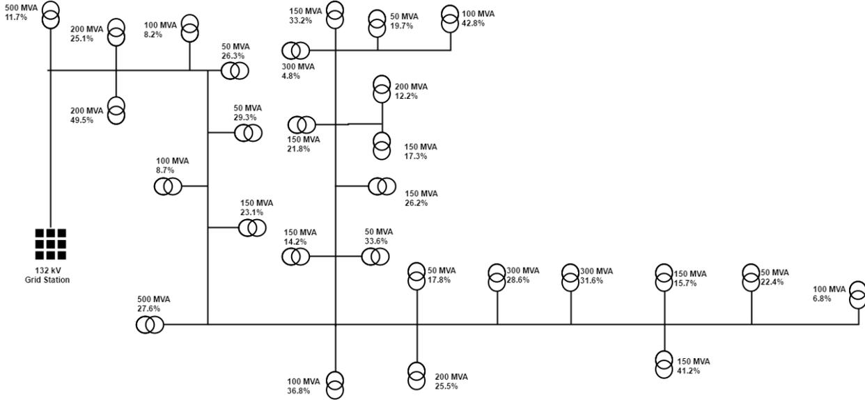
Fig. 2. 11 kV Dhari Distribution Feeder from 132 kV Larkana Grid Station
