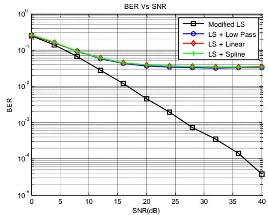
Fig. 6 Performance of OFDM system using BPSK for channel order 40
