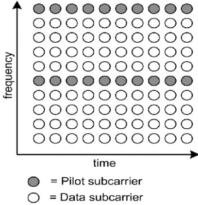
Fig. 3 Comb-type Channel Estimation
