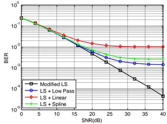
Fig. 5 Performance of OFDM system using BPSK for channel order 26
