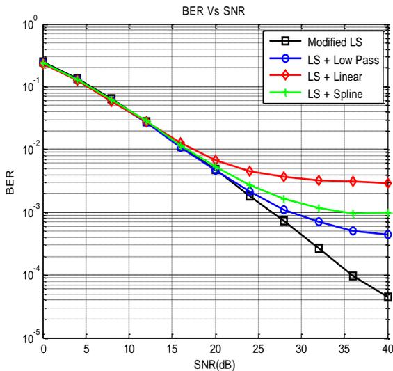
Fig. 4 Performance of OFDM system using BPSK for channel order 20
