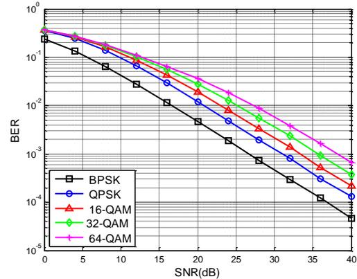
Fig. 7 Comparison curves of OFDM system using M-LS for different modulation schemes for channel order 20
