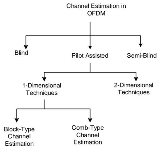
Fig. 2 Types of Channel Estimation
