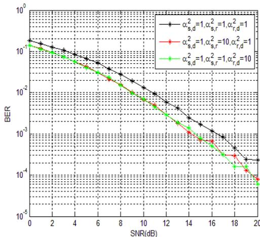
Fig. 3 Performance Analysis of Proposed AZF Protocol (BER vs SNR<sub>(dB)</sub>)
