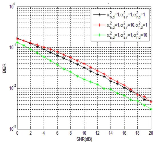
Fig. 2 Performance Analysis of AF Protocol (BER vs SNR<sub>(dB)</sub>)
