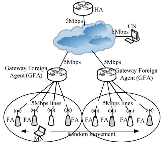
Fig.10. Network Topology of Proposed Method
