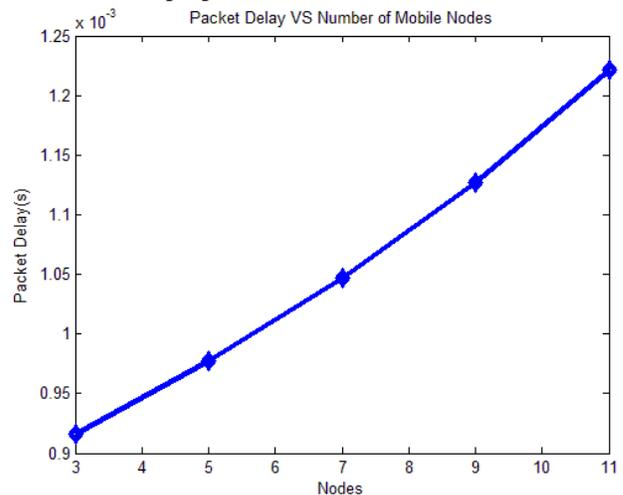
Fig.17. Packet Delay as a Function of Number of Mobile Nodes
