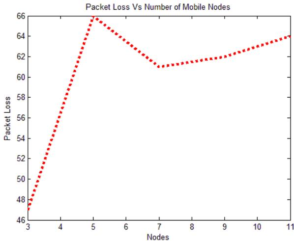
Fig.18. Packet Loss as a Function of Number of Mobile Nodes
