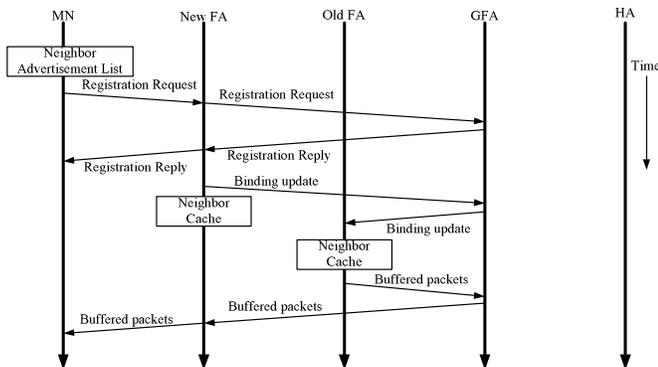
Fig.6. Signaling Diagram of the Proposed Method
