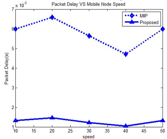
Fig.14. Packet Delay as Function of Mobile Nodes' Speed
