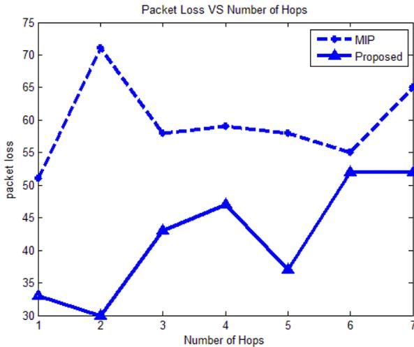
Fig.15. Packet Loss as a Function of Number of Hops
