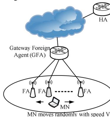
Fig.1. Networking Topology of Mobile IP Regional Registration with FOSH
