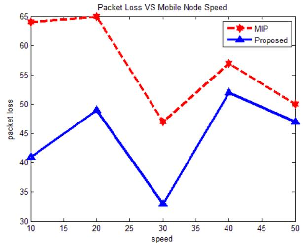
Fig.13. Packet Losses as Function of Mobile Nodes' Speed
