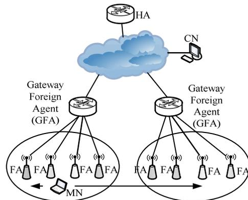
Fig.8. Hierarchical Topology of Proposed Method
