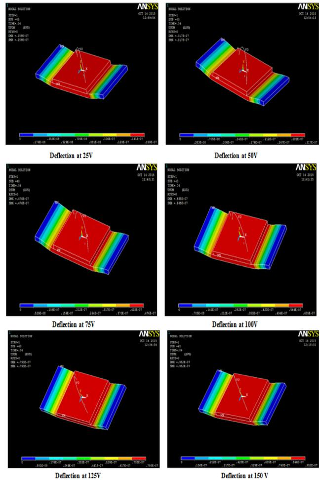
Fig. 2 Deflection at 25V, 50 V , 75 V , 100V , 125V , 150V
