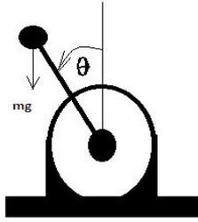
Fig. 1 Simple Inverted Pendulum system.
