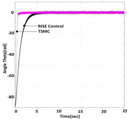
Fig. 3 Regulation of pendulum angle at zero rad.
