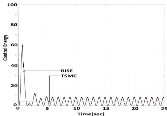
Fig. 6. Control Energy as function of time for RISE and TSMC.
