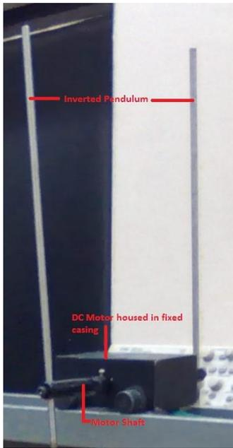
Fig. 2 Inverted Pendulum testbed.
