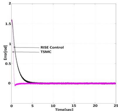
Fig. 4 Tracking error with RISE Control and TSMC.
