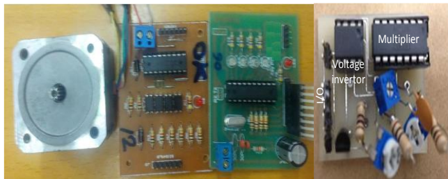
Fig. 5 Motor control unit (left side), transmitter module (right side)
