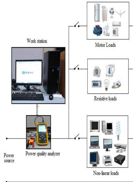
Fig. 1 Experimental setup with different loads
