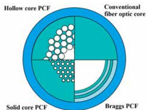
Fig. 5. A 4-in-1 logical diagram to show comparison of cores of 3 types of PCF and conventional fiber. White areas show air/vacuum areas while different colored areas indicate solid material with different refractive indices. Outermost rings shows conventional fiber cladding. (Not to scale!)
