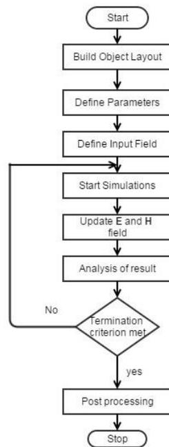
Fig. 4. Flow chart representing steps of numerical analysis of photonic crystals.
