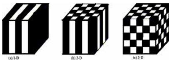
Fig. 3. Types of photonic crystals. (a) 1-D, (b) 2-D, (c) 3-D photonic crystals have periodicity in one-, two-, and three- dimensions respectively. Black and white colors in the figure respectively represent materials of high and low permittivity.
