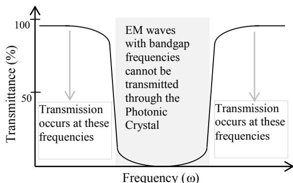
Fig. 2. Illustration of transmission spectrum of a PBG material. Transmission of EM waves at the bandgap frequencies are blocked by the photonic crystal.
