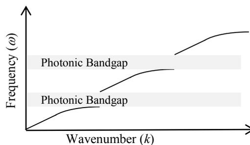
Fig. 1. An example of dispersion relation (i.e.  $\omega$ - $k$  relation) in arbitrary units of a PBG material. Bandgaps are indicated in the figure.
