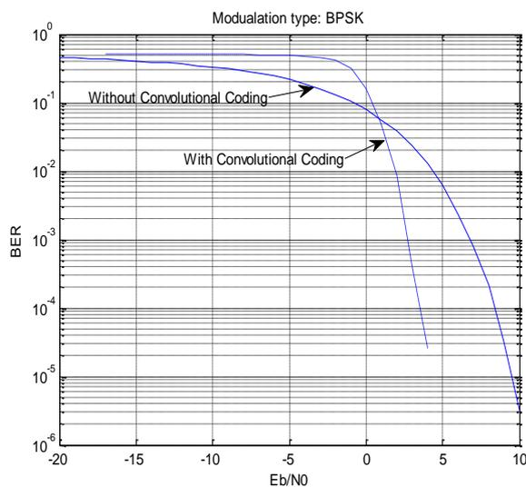
Fig. 1. BER vs  $E_b/N_0$  for Hamming Code and Convolutional Code.
