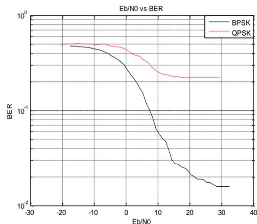
Fig. 2.  $E_b/N_0$  vs BER using BPSK, QPSK Modulation, Hamming code and interleaving.
